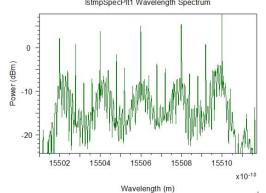
Fig 3.6 Optical spectrum at 50mW power with Unequal channel spacing
