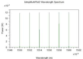
Fig 3.4 Clear view optical spectrum at 20mW power with Unequal channel spacing
