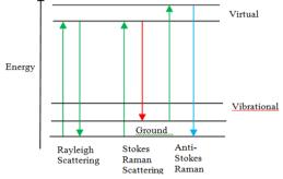
Fig. 2: Stokes and antistokes process
