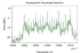
Fig 3.3 Clear view optical spectrum at 20mW power with equal channel spacing
