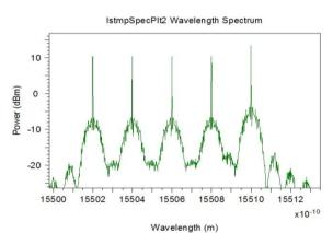
Fig 3.5 Optical spectrum at 50mW power with equal channel spacing IstmpSpecPltt Wavelength Spectrum
